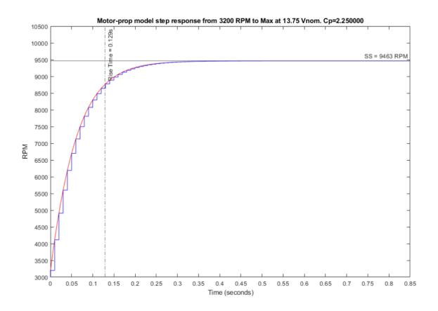
Model Step-reponse with Cp Adjusted to better match test stand output at steady-state
