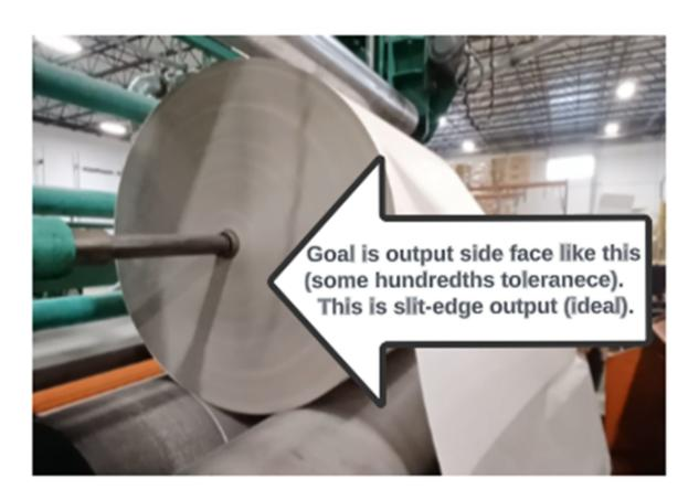
Some applications do not permit an edge trim and must regulate the input roll lateral position to maintain a degree of uniformity on the output roll face. For example, when slitting one roll into two with a single cutter in the middle with no cutters trimming a small waste strip on each side.
