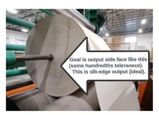
Some applications do not permit an edge trim and must regulate the input roll lateral position to maintain a degree of uniformity on the output roll face. For example, when slitting one roll into two with a single cutter in the middle with no cutters trimming a small waste strip on each side.
