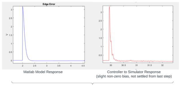
Good match of simulator response to production controller and matlab model. This indicates accurate implementation of plant model within the simulator as well as controller implementation.
