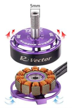
Draw up cool air from base and through the coils Higher efficiency and longer life.
